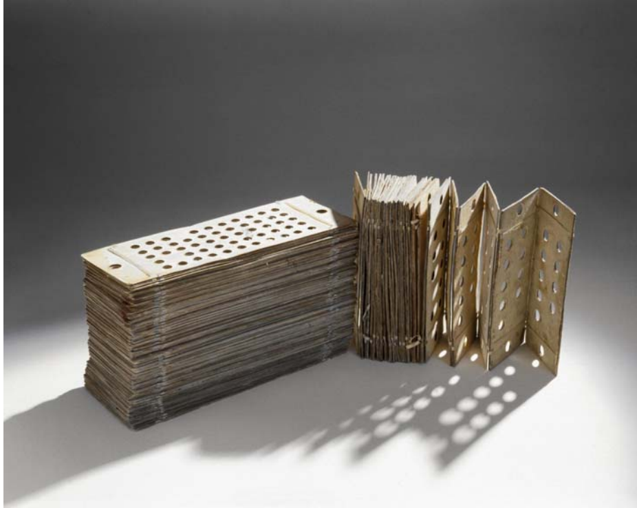
Perforation cards to be used with the Analytical Engine, c. 1879. Photo: Science Museum/SSPL
